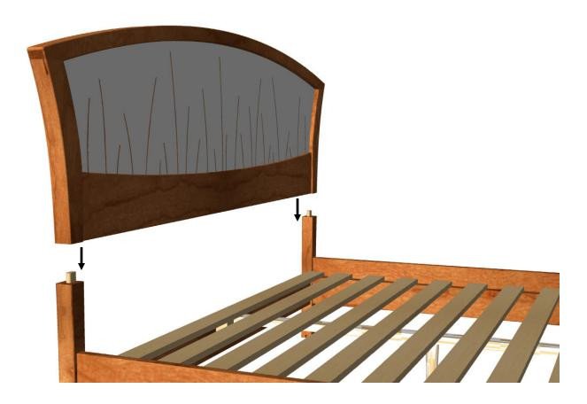
7. Connect the upper and lower headboard sections using the headboard connectors, screws and hex key:
