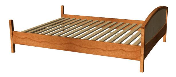
6. Place upper headboard onto the lower headboard, allowing the wooden pegs in the lower to fit into the holes in the upper:
