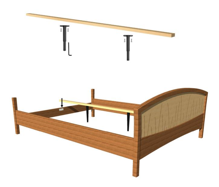
4. Adjust each metal adjustable foot by rotating the bottom half of the foot until it touches the floor.
