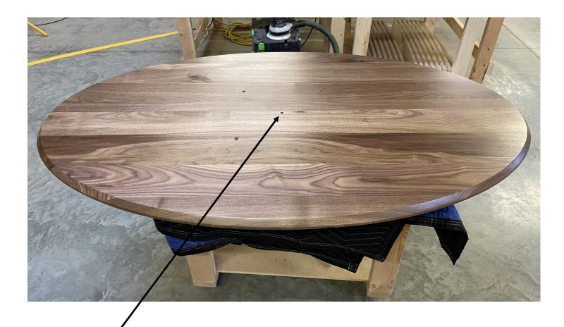
2. Note the hole in the center of the table top. In the next step the short dowel in the top of the base will drop into this hole, aligning the top and the base.
