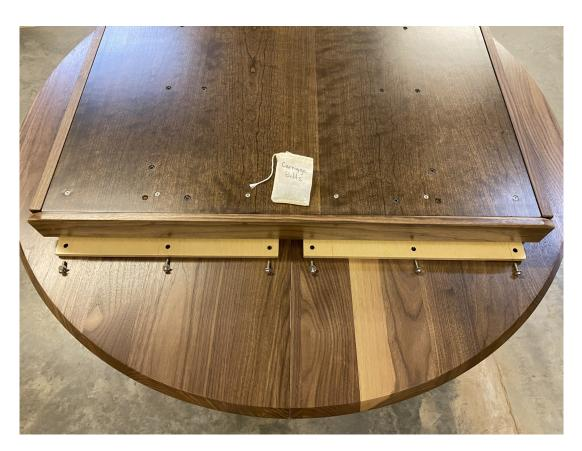
2) Attach the leg plates to the slide carriage using the leg screws. Fully tighten all of these bolts.
